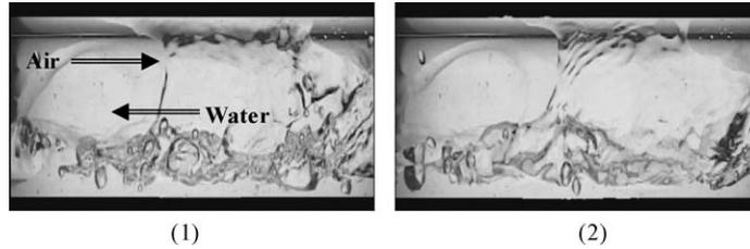
Fig. 12. Breakdown of the wave at the onset of flooding of  $Re_L = 540$ ,  $Re_G = 6704$  and  $\theta = 60^\circ$  (frame interval was 1/30 s).
