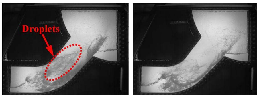
Fig. 8. Interfacial behaviour of air–water in hot leg channel during flooding (air–water,  $\dot{m}_L = 0.30$  kg/s and  $\dot{m}_G = 0.25$  kg/s).
