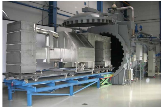
Fig. 3. Hot leg model at the TOPFLOW test facility.
